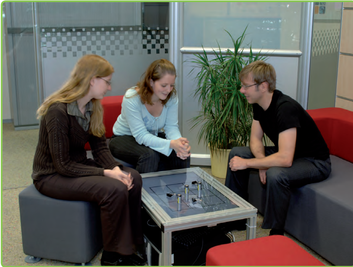
Figure 3: The "Interactive Table" Contains an interactive Tic Tac Toe Game; Arbitrary Objects of Everyday Life are Automatically Recognized and Assigned to Players
